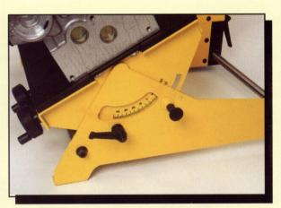
The table is adjustable  $45^{\circ}$  to the front and  $30^{\circ}$  to the back side.
