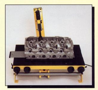
The post is adjustable  $0^{\circ}$  to  $25^{\circ}$  to both sides.
