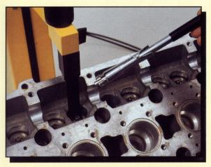
The valve keepers are easy to remove and replace, thanks to the open design of the pressure foot.
