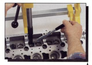
The valve keepers are easy to remove and replace, thanks to the open design of the pressure tool.
