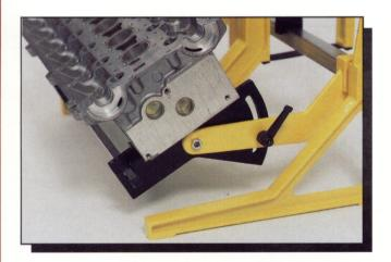
The angle of the head support is adjustable.
